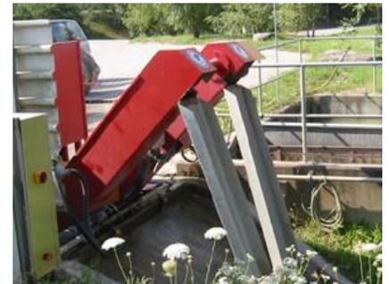
The scraper conveyors are automatically carrying out the dewatered sludge.
