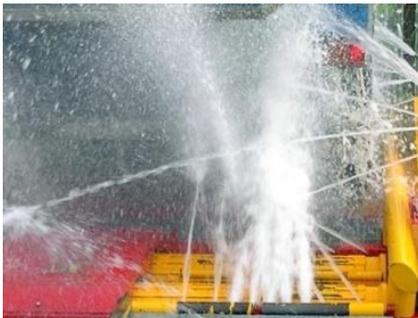
Simultaneous and Intensive washing of the dual back axles with the megawash option.
